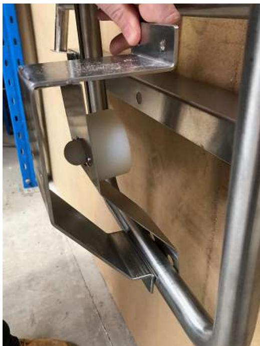
4. The wall bracket should be positioned as per image below where the top of the wall bracket meets that main seat support bar.
